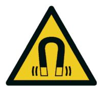
A WARNING Magnetic field. Could cause interference with pacemakers or other medical devices. Metal objects could become pinch points. Stand clear.
