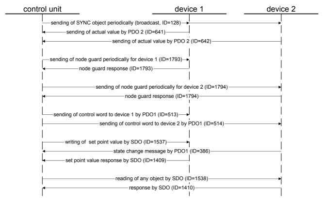
To be observed: Messages with a low identifier are transmitted with higher priority. So a PDO message may be transmitted between SDO request and SDO response.
