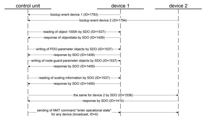
With the PDO parameters it is determined which objects are contained in the PDO and when the latter will be transmitted. The transmission can be e.g. event-driven (i.e. in case of an alteration of the object contained in the PDO), or cyclically (e.g. after every fifth SYNC message).
