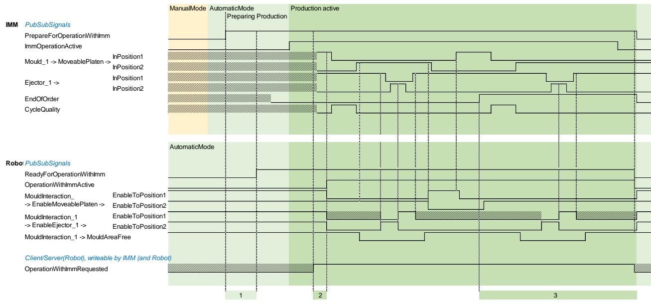
**Figure 12 – Example timing diagram for starting and ending of interaction in automativ mode**
