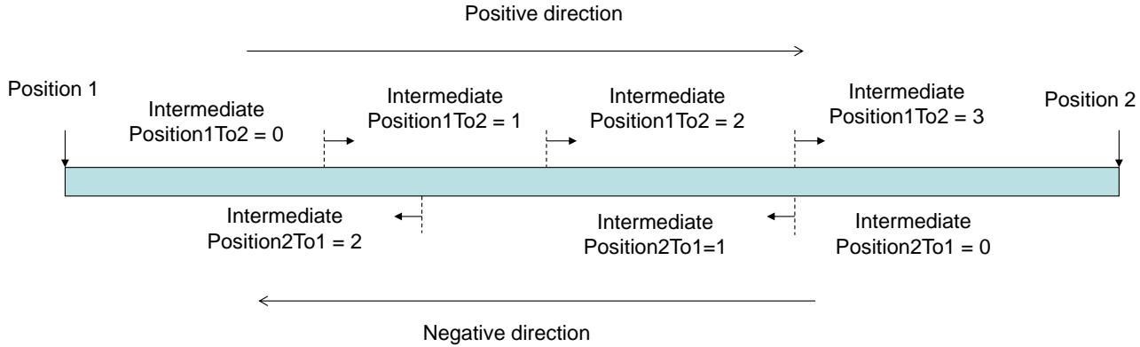
**Figure 4 – Definition of intermediate positions signals**
