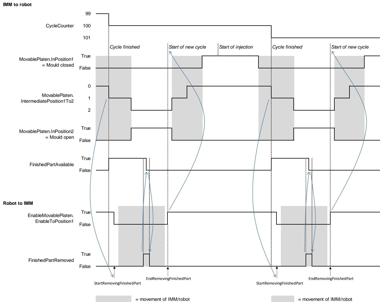
**Figure 6 – Example for timing for signals for part tracking (robot starts movement during mould opening)**
