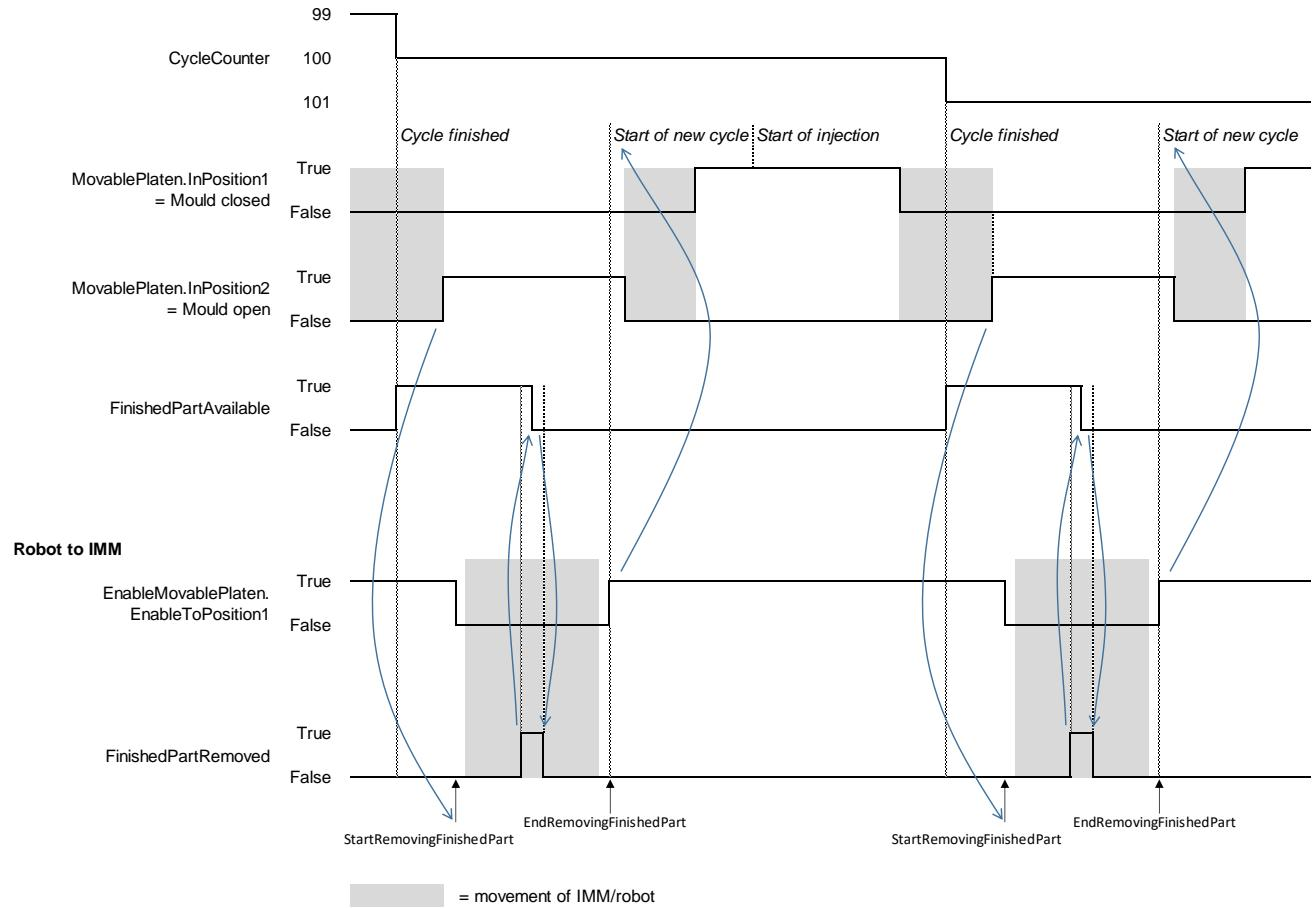
**Figure 5 – Example for timing for signals for part tracking (robot waits for full mould opening)**
