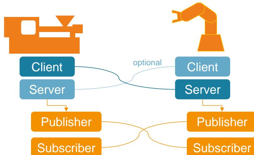
**Figure 1 – Combination of Client-Server and PubSub communication**
