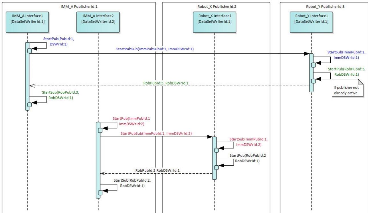
**Figure 8 – Example for StartPubSub for 1 IMM with 2 robots**
